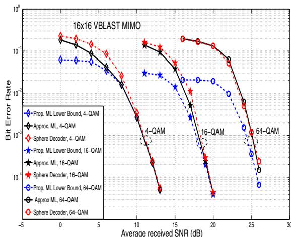
Fig. 2. Comparison of the proposed lower bound on ML performance for  $n = 1$  and the 'approximate ML' performance with the ML performance predicted by sphere decoder for  $16 \times 16$  V-BLAST MIMO with 4-QAM, 16-QAM, and 64-QAM.
