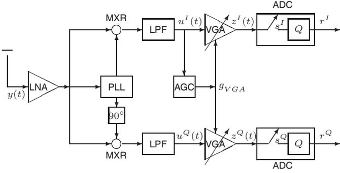
Fig. 1. Receiver analog front end (AFE) .
