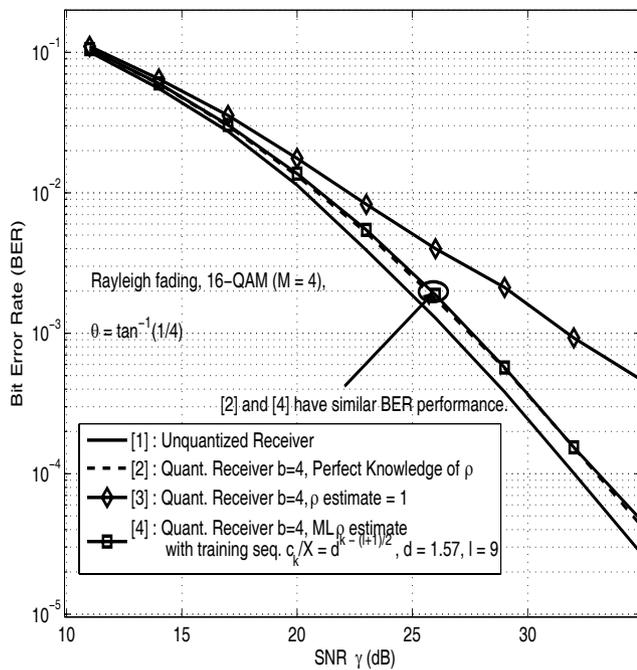
Fig. 10. BER performance with a quantized receiver ( $b = 4$ ) and imperfect receiver knowledge of  $\rho$ . Rotated 16-QAM ( $M = 4$ ).
