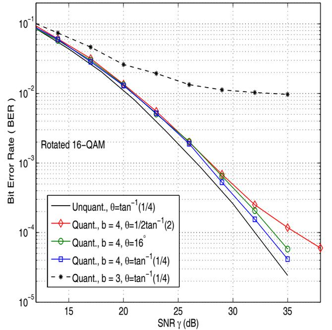
Fig. 7. BER vs. SNR for a quantized receiver.  $b = 4$ , 16-QAM and perfect channel state information at receiver.
