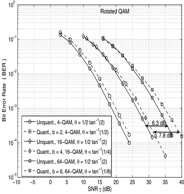
Fig. 8. BER comparison between quantized and unquantized receivers. 4-, 16-, 64-QAM. Perfect channel state information at receiver.
