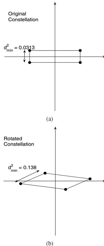
Fig. 3. Signal space of the received 2-D codewords. The gains along the horizontal and vertical signal component/dimension are  $|h_1| = 1$  and  $|h_2| = 1/4$  respectively.  $d_{\min}^2$  is the minimum Euclidean distance between any two received codewords.
