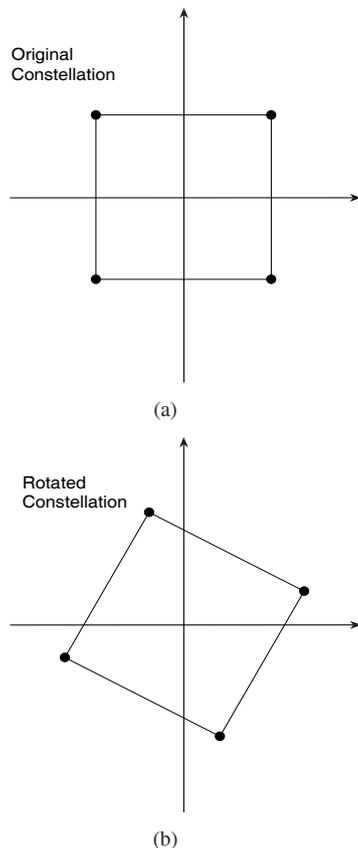
Fig. 2. Signal space of the transmitted constellation consisting of four codewords in 2 dimensions (horizontal and vertical). The average transmit power constraint is  $P_T = 1/4$ . For the rotated constellation, the rotation angle is  $28.5^\circ$ . The codewords are represented by solid dots.
