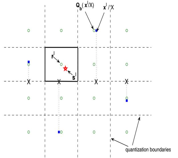
Fig. 5. Signal space at the quantizer input with  $b = 2$  (real component). Rotated 4-QAM ( $\theta = 20^\circ$ ) depicted with dark filled squares.
