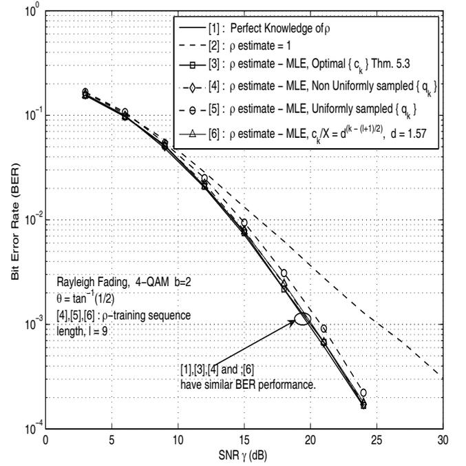
Fig. 9. BER performance with a quantized receiver ( $b = 2$ ) and imperfect receiver knowledge of  $\rho$ . Rotated 4-QAM ( $M = 2$ ).
