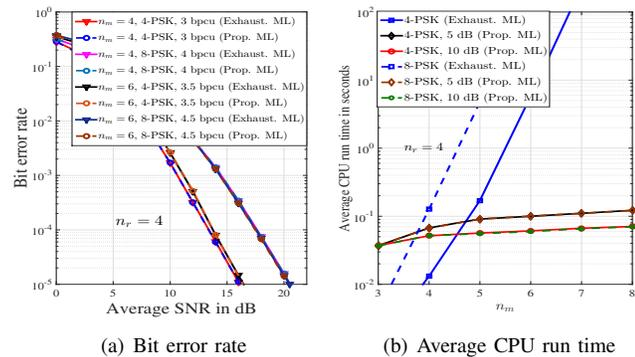
Fig. 2. BER and CPU run time comparison between the proposed low-complexity ML detector and the exhaustive search ML detector.
