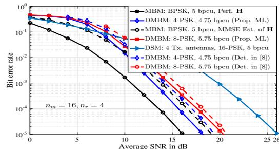
Fig. 3. BER comparison between DMBM, DSM, and MBM with  $n_r = 4$ .
