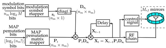
Fig. 1. Differential MBM transmitter.
