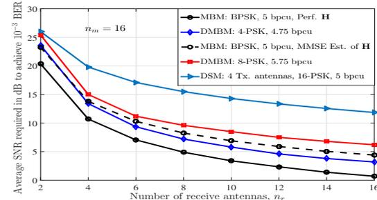
Fig. 4. Average SNR required to achieve  $10^{-3}$  BER as a function of  $n_r$  for DMBM, DSM, and MBM.
