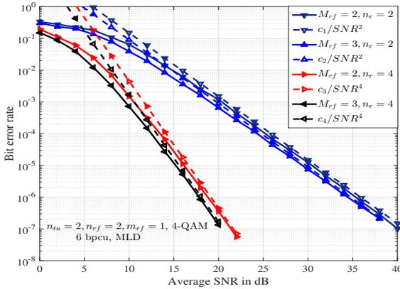
Fig. 9. Diversity orders achieved by MI-based MAP selection in MIMO-MBM with  $n_{tu} = n_{r,f} = 2, m_{r,f} = 1, 4\text{-QAM}$ , and 6 bpcu for various values of  $M_{r,f}$  and  $n_r$ : i)  $M_{r,f} = 2, n_r = 2$ ; ii)  $M_{r,f} = 3, n_r = 2$ ; iii)  $M_{r,f} = 2, n_r = 4$ ; iv)  $M_{r,f} = 3, n_r = 4$ .
