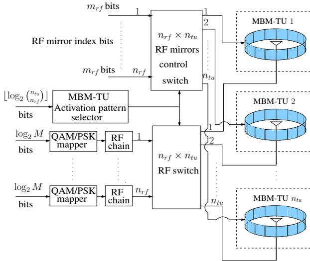
Fig. 2. GSM-MBM transmitter.
