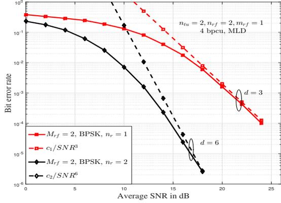
Fig. 8. Diversity orders achieved by ED-based MAP selection in MIMO-MBM for various system parameters.
