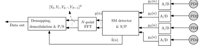
Fig. 3. Proposed I-NDC OFDM receiver.
