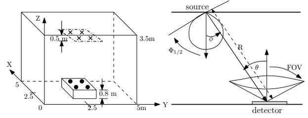
Fig. 4. Geometric set-up of the considered indoor VLC system. A dot represents a photo detector and a cross represents an LED.
