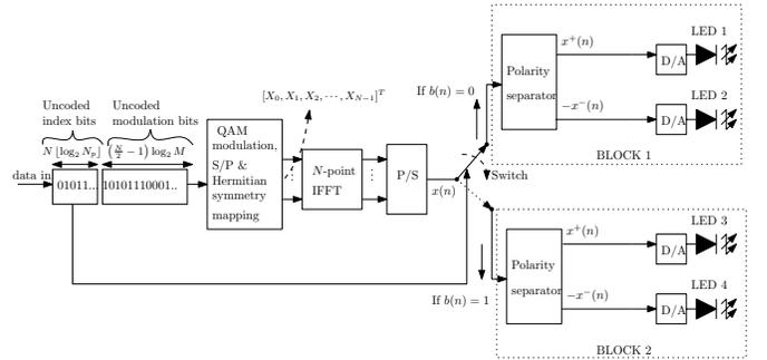
Fig. 2. Proposed I-NDC OFDM transmitter.
