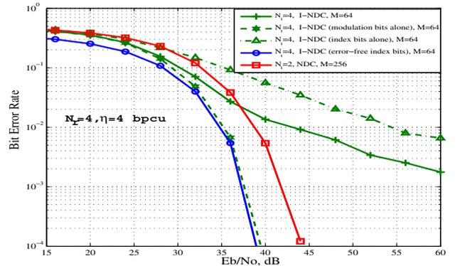
Fig. 6. Reliability of modulation bits and index bits in the proposed I-NDC OFDM for  $\eta = 4$  bpcu,  $N_r = 4$ .
