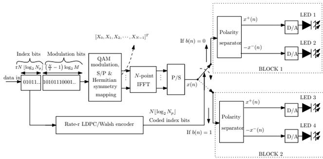
Fig. 7. Proposed CI-NDC OFDM transmitter.
