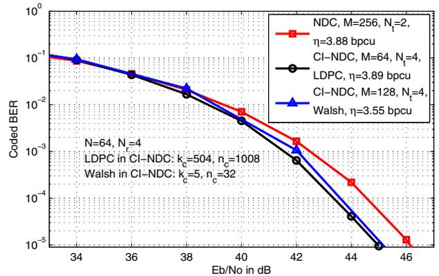
Fig. 9. BER performance of the proposed CI-NDC OFDM and NDC OFDM at  $\eta = 3.8$  bpcu,  $N_r = 4$ .
