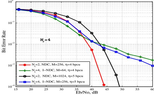
Fig. 5. Comparison of the BER performance of NDC OFDM and the proposed I-NDC OFDM for  $\eta = 4, 5$  bpcu,  $N_r = 4$ .
