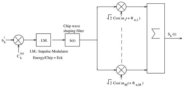
Fig. 1. Multicarrier DS-CDMA Transmitter of  $k$ th user
