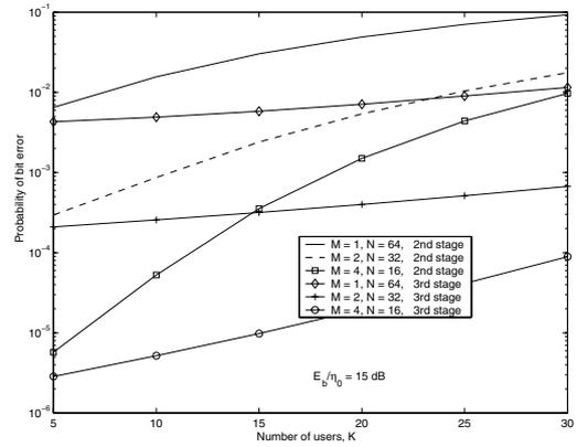
Fig. 5. Probability of bit error,  $P_e$ , versus number of users,  $K$ , at different stages of the PIC for the uncoded system with different values of  $M$  ( $M = 1$ ,  $N = 64$ ;  $M = 2$ ,  $N = 32$ ;  $M = 4$ ,  $N = 16$ ). Analysis plots only.  $E_b/\eta_0 = 15$  dB.
