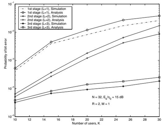
Fig. 7. Comparison of the analytical bounds on the coded BER versus the simulated BER at different PIC stages of the convolutionally coded system.  $R = 2$ ,  $M = 1$ ,  $N = 32$ ,  $E_b/\eta_0 = 15$  dB.
