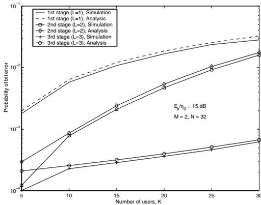
Fig. 4. Probability of bit error,  $P_e$ , versus number of users,  $K$ , at different stages of the PIC receiver for the uncoded system. Analysis and simulation plots.  $M = 2$ ,  $N = 32$ ,  $E_b/\eta_0 = 15$  dB.
