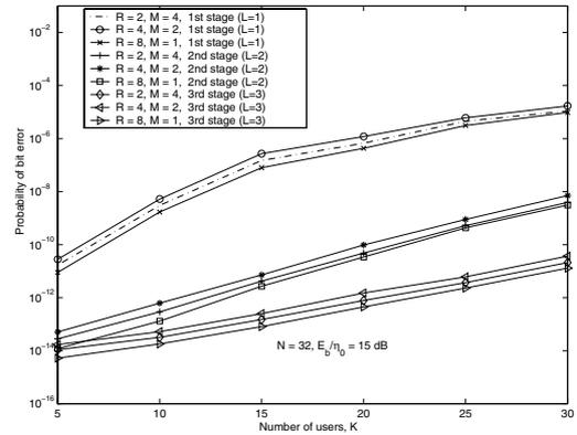
Fig. 6. Upper bound on the coded BER versus number of users,  $K$ , at different PIC stages of the convolutionally coded system with different combinations of code rate ( $1/R$ ) and number of subcarriers ( $M$ ).  $N = 32$ ,  $E_b/\eta_0 = 15$  dB.
