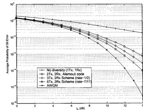
Fig. 6. BER performance of 16-QAM with different STBCs – *i*) 2 Tx antennas using rate-1 STBC (Alamouti code), *ii*) 3 Tx antennas using rate-1/2 STBC, *iii*) 5 Tx antennas using rate-7/11 STBC. Number of receive antennas,  $L_2 = 2$ .
