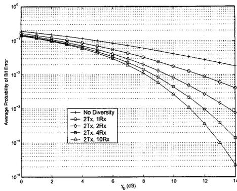
Fig. 3. BER performance of 16-QAM with 2 transmit antennas and  $L_r = 1, 2, 4, 10$  receive antennas using rate-1 STBC (Alamouti code).
