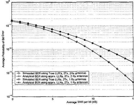
Fig. 2. Comparison of the analytical BER evaluated using approximate LLRs vs the simulated BER using the LLRs without approximation. 16-QAM with rate-1 STBC (Alamouti code). 2Tx/2Rx and 2Tx/1Rx antennas.
