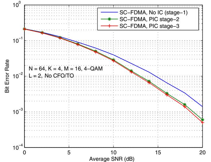
Fig. 2. BER performance of SC-FDMA without and with IC cancellation.  $N = 64$ ,  $K = 4$ ,  $M = 16$ ,  $L = 2$ , 4-QAM, No CFO and TO. IC removes residual interference and improves performance.
