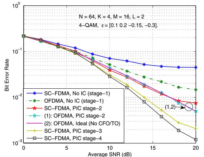
Fig. 3. Comparison of BER performance between SC-FDMA and OFDMA with CFO.  $N = 64$ ,  $K = 4$ ,  $M = 16$ ,  $L = 2$ ,  $\epsilon = [0.1, 0.2, -0.15, -0.3]$ . No TO. User 1 is desired user. SC-FDMA (without IC) performs worse than OFDMA in the presence of CFO. With the proposed PIC, however, SC-FDMA recovers its frequency diversity advantage and outperforms OFDMA.
