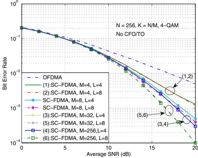
Fig. 1. Comparison of uncoded BER performance of SC-FDMA and OFDMA with no CFO and TO.  $N = 256$ ,  $M = 4, 8, 32, 256$ ,  $K = N/M$ ,  $L = 4, 8$ , 4-QAM, and interleaved allocation, SC-FDMA outperforms OFDMA due its frequency diversity advantage.
