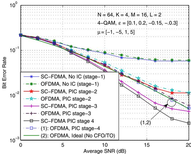
Fig. 4. Comparison of BER performance between SC-FDMA and OFDMA with CFO and TO.  $N = 64$ ,  $K = 4$ ,  $M = 16$ ,  $L = 2$ ,  $\epsilon = [0.1, 0.2, -0.15, -0.3]$ ,  $\mu = [-1, -5, 1, 5]$ . User 1 is desired user. With the proposed PIC, SC-FDMA recovers its frequency diversity advantage and outperforms OFDMA.
