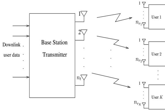
Fig. 1. Multiuser MIMO downlink system.
