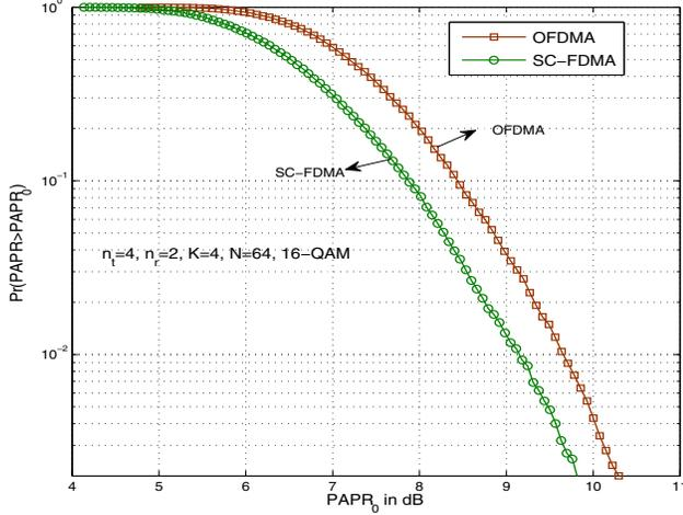
Fig. 5. PAPR performance of multiuser MIMO SC-FDMA and OFDMA for  $n_t = 4, n_r = 2, K = 4, N = 64, 16\text{-QAM}$ .
