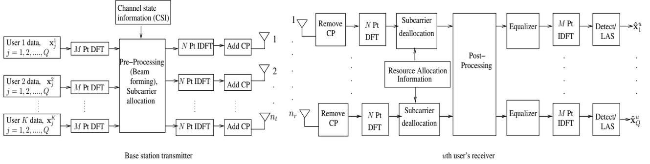
Fig. 2. Transmitter and receiver block diagrams of MIMO SC-FDMA on the downlink.
