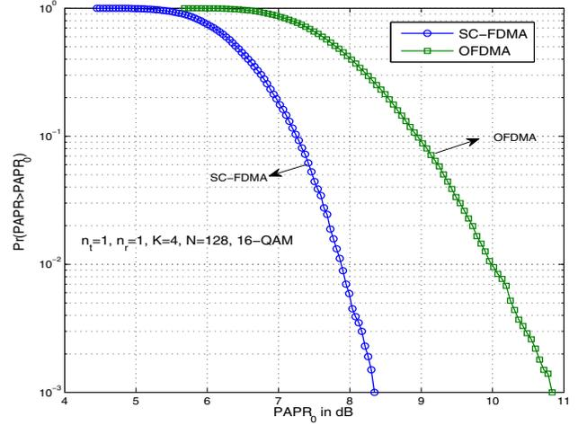
Fig. 3. PAPR performance of multiuser SISO SC-FDMA and OFDMA for  $n_t = 1, n_r = 1, K = 4, N = 128$ , 16-QAM.
