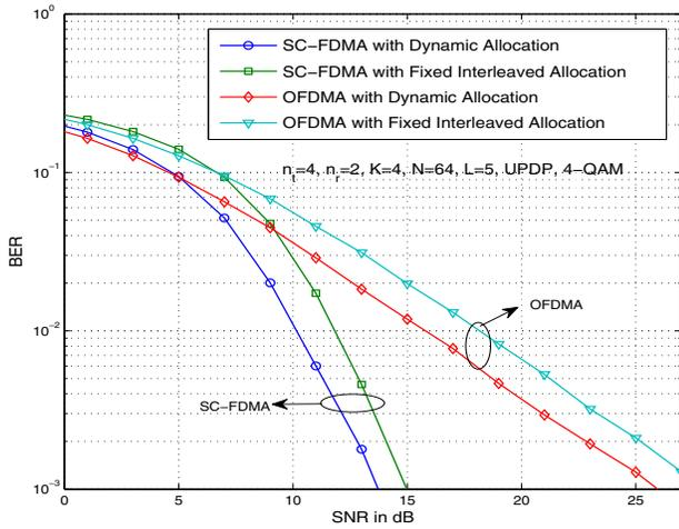
Fig. 6. BER performance of multiuser MIMO downlink SC-FDMA and OFDMA for  $n_t = 4, n_r = 2, K = 4, N = 64, L = 5, 4\text{-QAM}$ .
