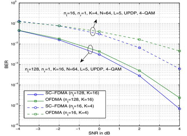
Fig. 8. BER performance of large-scale multiuser MISO downlink SC-FDMA and OFDMA for *i*)  $n_t = 16, n_r = 1, K = 4, L = 5, 4\text{-QAM}$ , and *ii*)  $n_t = 128, n_r = 1, K = 16, L = 5, 4\text{-QAM}$ .
