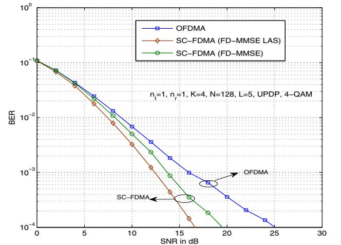
Fig. 4. BER performance of multiuser SISO downlink SC-FDMA and OFDMA for  $n_t = 1, n_r = 1, K = 4, N = 128, L = 5$ , 4-QAM.
