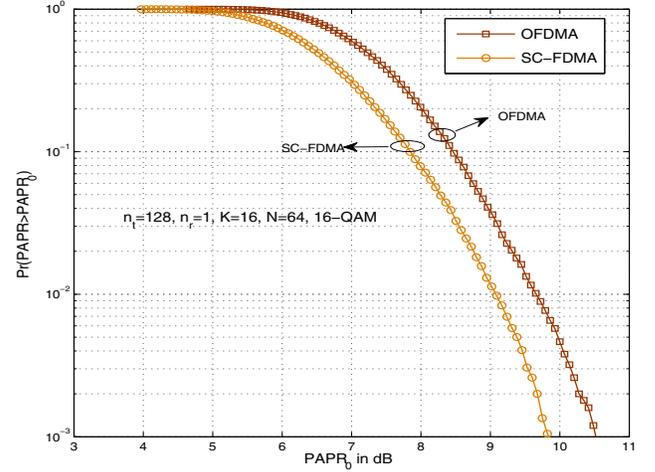
Fig. 7. PAPR performance of large-scale multiuser MISO SC-FDMA and OFDMA for  $n_t = 128, n_r = 1, N = 64, K = 16, 16\text{-QAM}$ .
