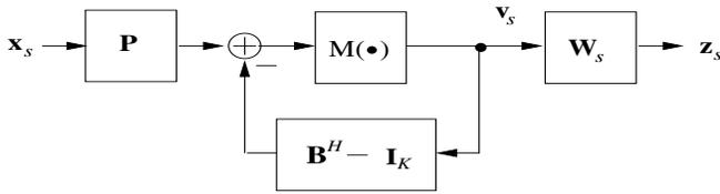
Fig. 2. Proposed THP precoder at the SBS with interference constraints.
