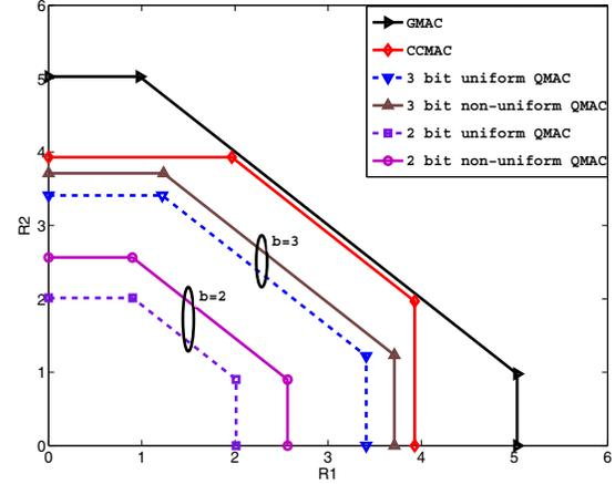
Fig. 6. Comparison between the achievable rate regions with uniform and non-uniform receiver quantization for a two-user MAC. User 1 uses a 16-QAM signal set and User 2 uses the optimally rotated 16-QAM. SNR per user = 15 dB.
