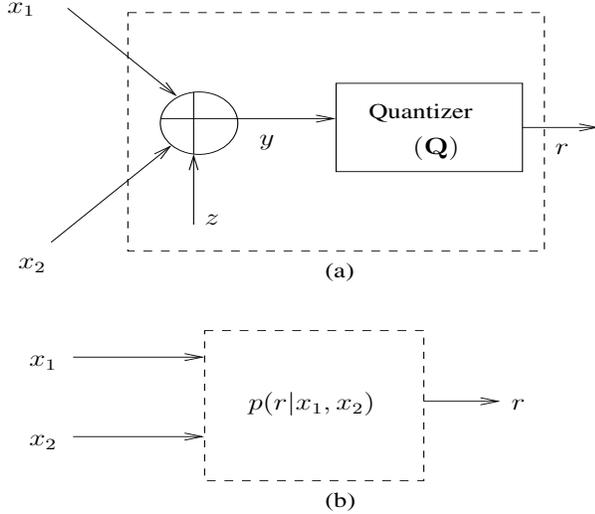
Fig. 1. (a) Two-user Gaussian MAC model with quantized output (b) Equivalent DMC.
