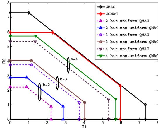
Fig. 5. Comparison between the achievable rate regions with uniform and non-uniform receiver quantization for a two-user MAC. User 1 uses a 64-QAM signal set and User 2 uses the optimally rotated 64-QAM. SNR per user = 22 dB.
