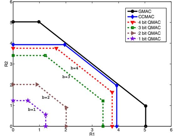
Fig. 2. Rate region of two-user QMAC with uniform quantizer. User 1 transmits from 16-QAM signal set, and User 2 transmits from an optimally rotated version of the first user's signal set. SNR per user = 15 dB.
