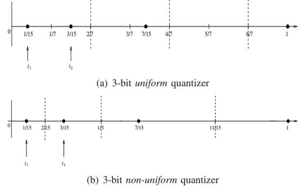
Fig. 4. Plot of the quantization intervals for 3-bit uniform and non-uniform quantizers. The boundaries between the quantization regions are demarcated by the dotted lines and the black dots show the points given in (23). Since the quantizer is symmetric about the origin, only the positive side is shown.
