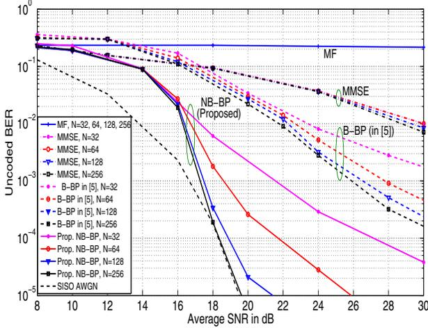
Fig. 3. Comparison of uncoded BER performance of the proposed NB-BP scheme with those of B-BP in [6], MMSE and MF detectors for  $N = 32, 64, 128, 256$ ,  $\alpha = 1$ , and 16-QAM.
