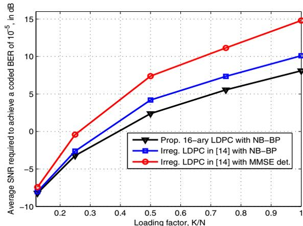
Fig. 6. Performance comparison of the proposed irregular non-binary LDPC codes with other LDPC codes for  $n = 1000$  coded symbols and 16-QAM.  $N = 128$  for different loading factors.
