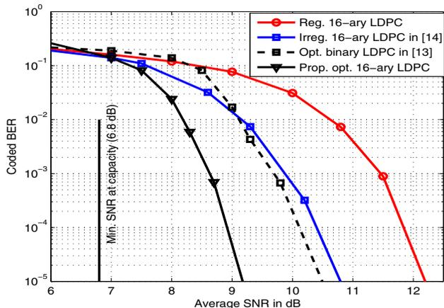
Fig. 5. Performance comparison of the proposed irregular non-binary LDPC codes with other LDPC codes for  $n = 1000$  coded symbols, 16-QAM and  $N = K = 64$ , at a spectral efficiency of 128 bits/s/Hz.
