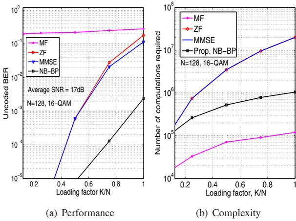
Fig. 4. Comparison of uncoded BER performance and complexity of the proposed NB-BP scheme with those of linear detectors (MMSE, ZF, MF) as a function of loading factor  $\alpha$ , with  $N = 128$  and 16-QAM.
