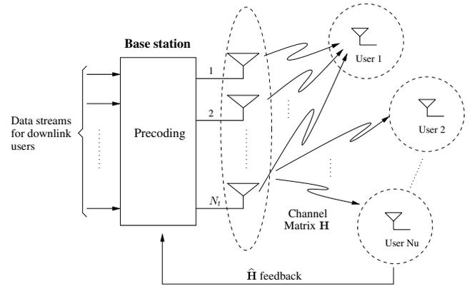
Fig. 1. Multiuser MIMO system on the downlink.
