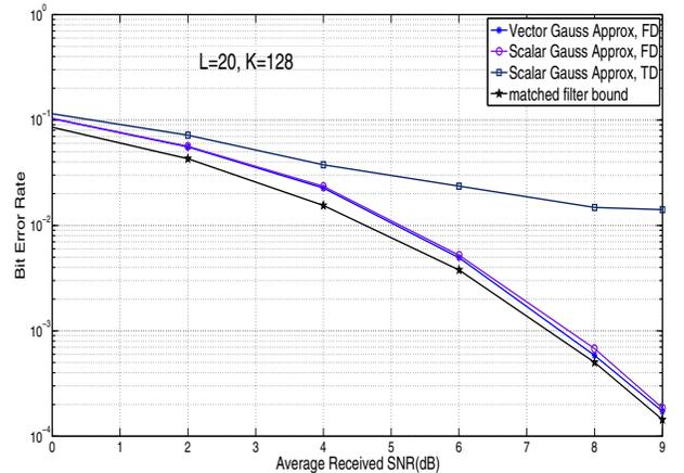
Fig. 2. Uncoded BER performance in single-input single-output CPSC system with  $L = 20, K = 128$ , uniform power delay profile: i) vector approximation approach in FD, 5 iterations, ii) scalar approximation approach in FD, 5 iterations, iii) scalar approximation approach in TD, 5 iterations, and iv) performance of matched filter receiver with no ISI, BPSK.
