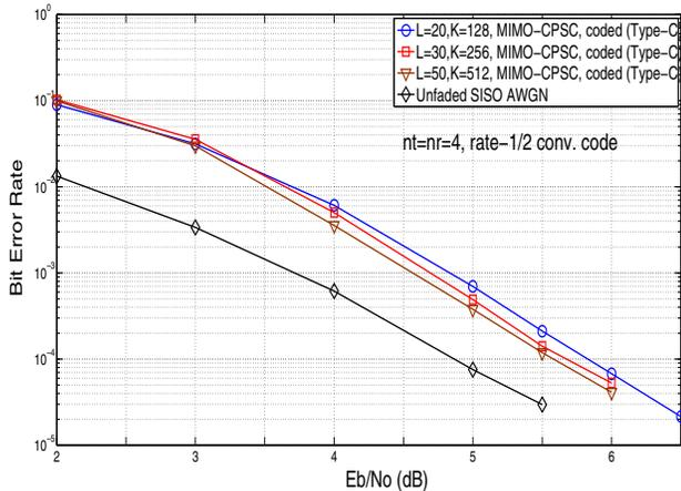
Fig. 4. Coded BER performance of turbo equalization in MIMO-CPSC system with  $n_t = n_r = 4$ , ( $L = 20$ ,  $K = 128$ ), ( $L = 30$ ,  $K = 256$ ), and ( $L = 50$ ,  $K = 512$ ). Uniform power delay profile.
