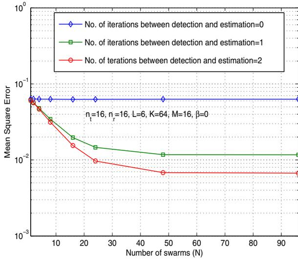
Fig. 4. Mean square error of iterative CPSO channel estimation as a function of number of swarms  $N$  for  $n_t = 16$ ,  $n_r = 16$ ,  $L = 6$ ,  $\beta = 0$ ,  $K = 64$ ,  $M = 16$  and SNR = 12 dB.
