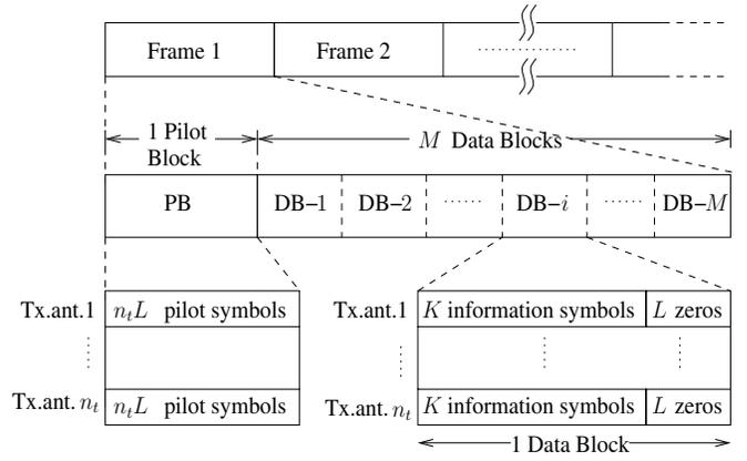
Fig. 1. Frame structure for MIMO-ZPSC system.
