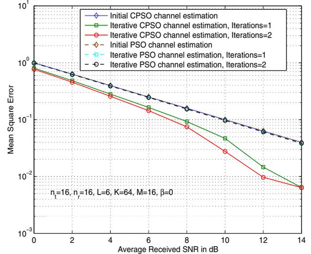
Fig. 2. MSE performance of CPSO/PSO channel estimation for different number of iterations between channel estimation and detection for  $n_t = 16$ ,  $n_r = 16$ ,  $\beta = 0$ ,  $L = 6$ ,  $K = 64$ ,  $M = 16$ .
