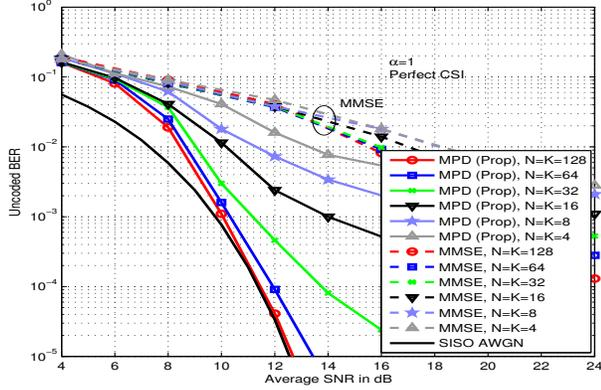
Fig. 5. Uncoded BER performance of the MPD algorithm and the MMSE detector for  $N = K = 4, 8, 16, 32, 64, 128$ .
