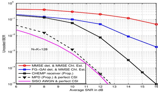
Fig. 7. Comparison of the BER performance of the proposed CHEMP receiver with those of 1) MMSE detector with MMSE channel estimate, and 2) FG-GAI detector in [6] with MMSE channel estimate, for  $N = K = 128$ .
