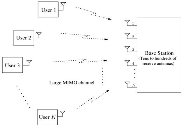
Fig. 1. Large-scale multiuser MIMO system model on the uplink.
