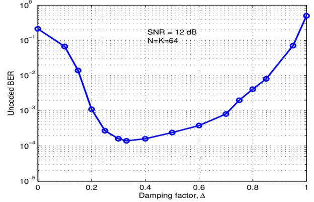
Fig. 4. Un-coded BER performance of the proposed MPD algorithm as a function of damping factor  $\Delta$ .  $N = K = 64$ , SNR=12 dB.
