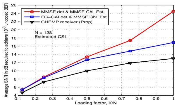
Fig. 8. Comparison between the average SNR required to achieve an uncoded BER of  $10^{-3}$  in 1) proposed CHEMP receiver, 2) MMSE detector with MMSE channel estimate, and 3) FG-GAI detector in [6] with MMSE channel estimate, at different loading factors with  $N = 128$ .
