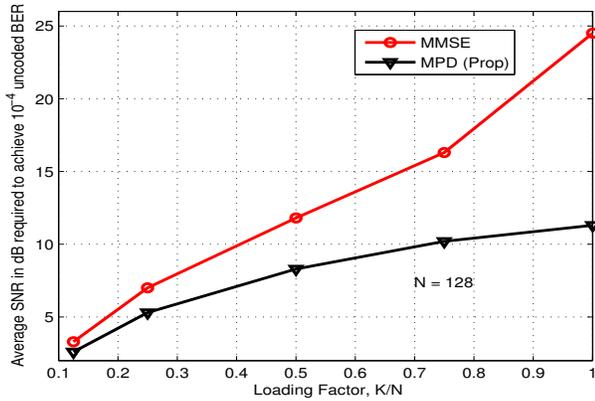
Fig. 6. Comparison between the average SNR required to achieve an uncoded BER of  $10^{-4}$  in MMSE detection and MPD at different loading factors with  $N = 128$ .
