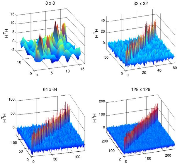
Fig. 2. Magnitude plots of  $\mathbf{H}^T \mathbf{H}$  for  $8 \times 8$ ,  $32 \times 32$ ,  $64 \times 64$ , and  $128 \times 128$  MIMO channels.
