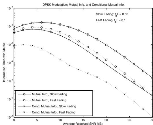
Fig. 2. Average MI,  $I(\beta_i; \beta_{i-1})$ , and conditional average MI,  $I(\beta_i; \beta_{i-2} | \beta_{i-1})$ , of the channel error process  $\beta_i$  with binary DPSK modulation on time-correlated Rayleigh fading channels.
